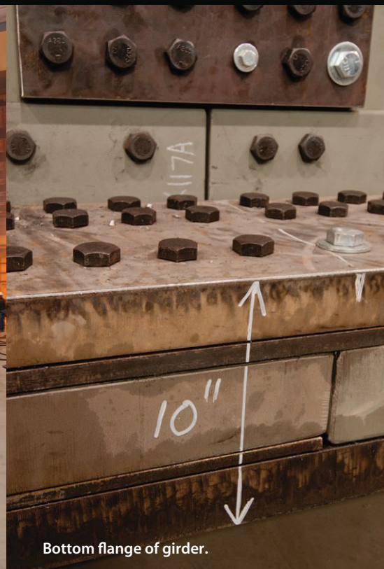
80-foot long railroad girder with bolt holes drilled zero to 80 feet within 1/32-inch.
